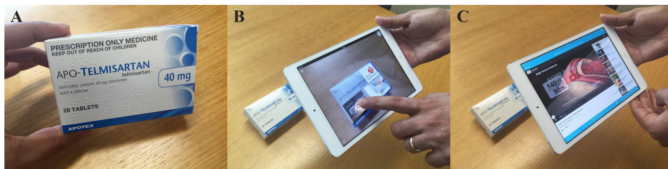
Figure 1 An example of how the augmented reality solution in this study works: Users install specific apps and scan predefined patterns (eg, package of a medicine) via their smartphone or tablet. These patterns, technically called 'triggers', initiate the retrieval and visualisation of digital content as overlaid information. (A) An ordinary package of telmisartan, a frequently prescribed angiotensin II receptor blocker. (B) The same package, augmented by the 'Layar' app. The app retrieves extra digital information and conveniently overlays it on top of the package; a clickable YouTube video about high blood pressure, a link to the Heart Foundation's website about medication management of high blood pressure and a flip-through slideshow of the most common side effects of telmisartan are shown. (C) YouTube video is shown instantly after user clicks on its thumbnail. (Photo credit: Dr Kara Burns. Patient consent for photography taken by Professor Lisa Nissen)
