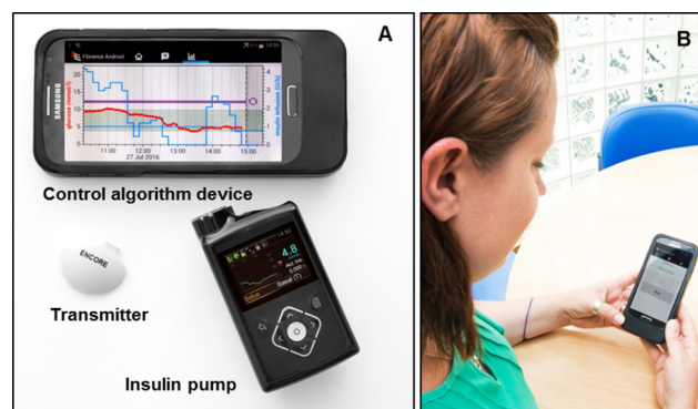
Figure 2 Closed-loop system prototype. (A) Components of the FlorenceM closed-loop system consist of a continuous glucose monitoring (CGM) transmitter with Enlite 3 sensor, an insulin pump (modified 640G pump) integrated with the CGM receiver and a mobile phone running the control algorithm. (B) A photo of a participant (obtained with consent) using the closed-loop system.
