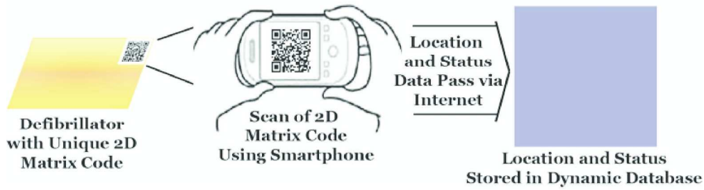
Figure 1: Use of Unique Device Identifier for AED Surveillance
