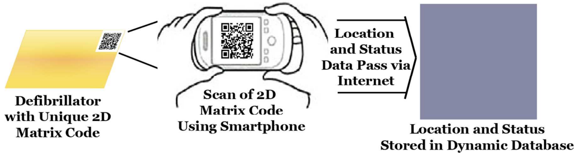
Figure 1: Use of Unique Device Identifier for AED Surveillance
