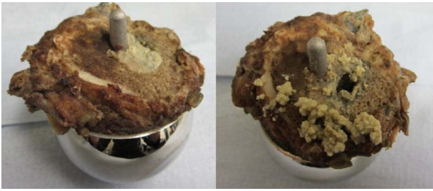
Figure 7 The femoral neck and prosthesis of a male patient in this study with a Birmingham Hip Resurfacing who was found to have blood cobalt of 155 µg/l on routine screening. He had no symptoms but elected for surgery 2 years later when he developed progressive discomfort in his hip. There were no obvious changes on plain x-rays. As can be seen on the right, there was a large cavity in the femoral neck filled with metal-stained, caseous material.
