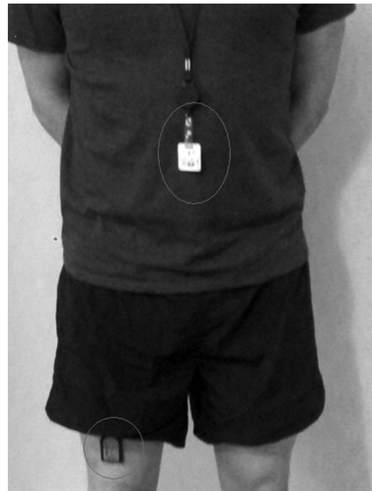
Figure 2 ActivPal accelerometer and radiofrequency identification tracking system to be worn by participants.
