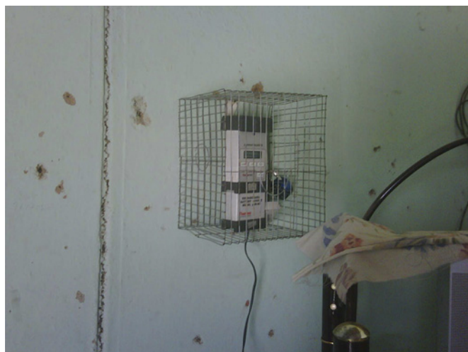
Figure 3 Particulate matter measurement device in place. pDR-1000 in place in study household, accompanied by HOBO Data Logger and protected by open cage for air flow.
