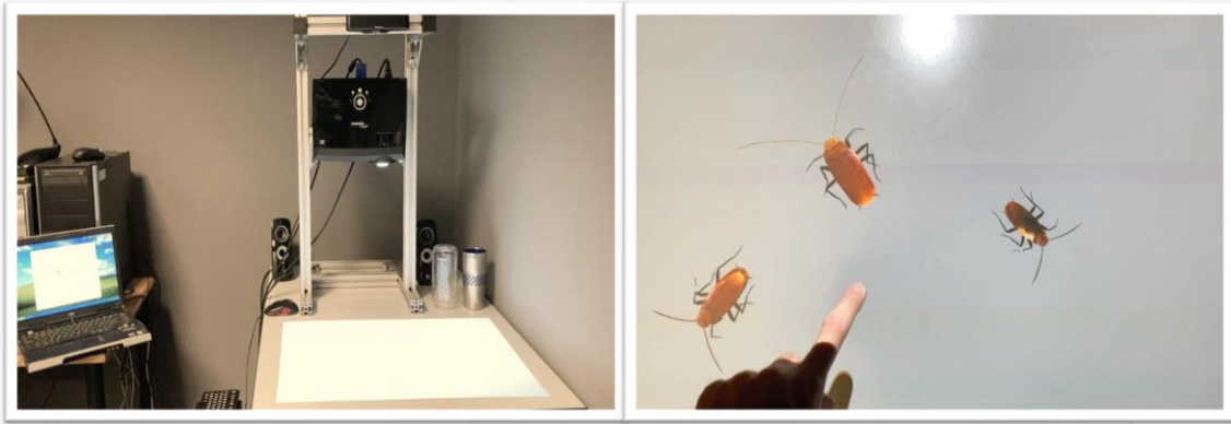
Figure 2. Images depicting the P-ARET system and an example of how the cockroaches looks like from the patient's view.
