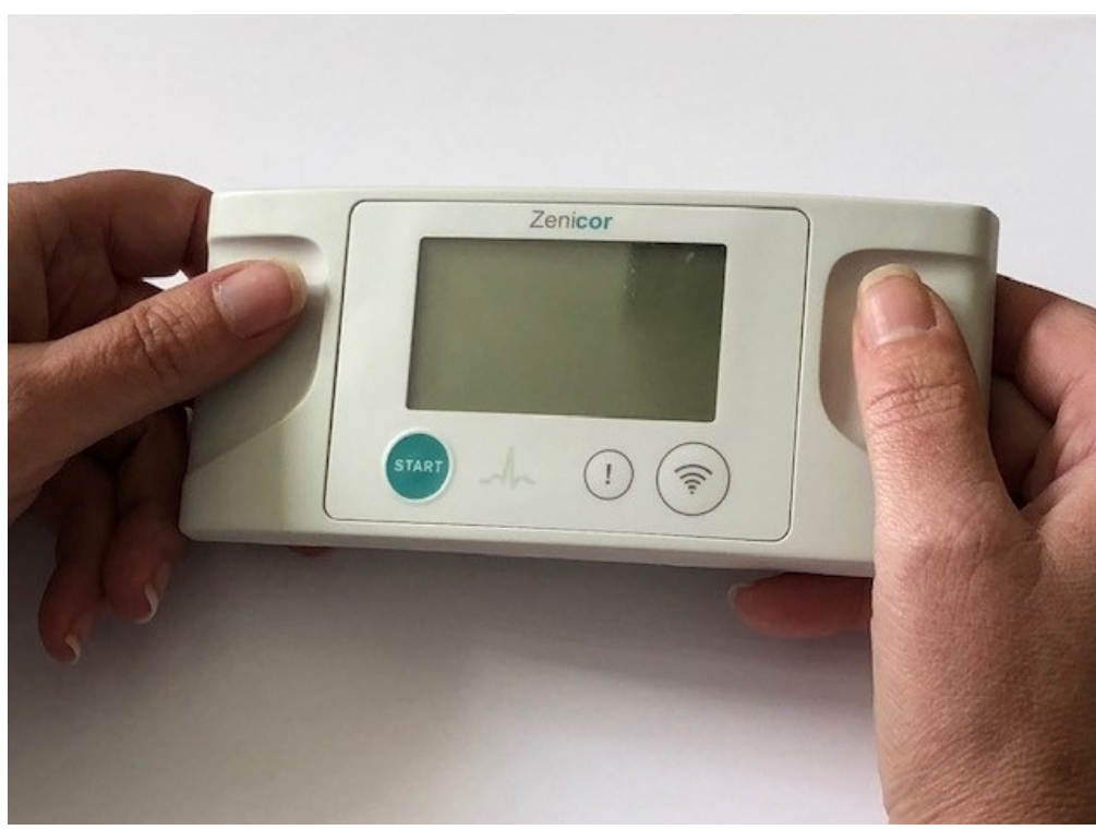
Figure 2. Zenicor hand-held ECG device used to screen for AF in the SAFER trial 225x167mm (72 x 72 DPI)
