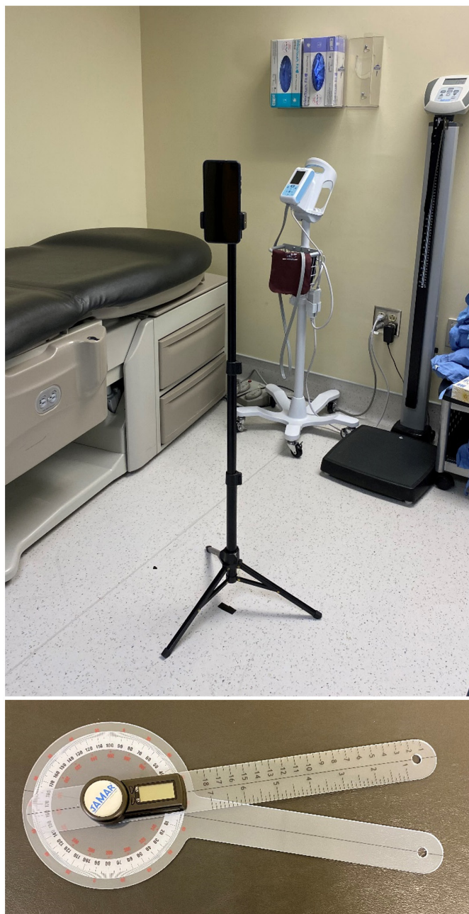
Figure 1 A mobile phone camera mounted on a TRIPOD (top) will be used to record videos of the joint hypermobility assessments. A 12.5" JAMAR Plus+clinical-grade digital goniometer (bottom) will be used to measure the range of motion at each joint. TRIPOD, Transparent Reporting of a multivariable prediction model for Individual Prognosis or Diagnosis.
