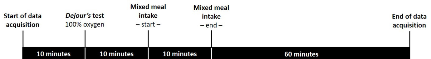
Figure 2 Data acquisition protocol. Heart rate, respiratory rate (RR), peripheral oxygen saturation (SpO 2 ) and circulating glucose values will be assessed using the CBmeter prototype. Heart rate will be computed from the ECG signal using a single-lead differential bipolar sensor (biosignalsplux SENSPRO-ECG1-30-30-30). RR will be measured using respiratory inductance plethysmography sensor (biosignalsplux SENSADV-RIP1); peripheral oxygen saturation will be assessed through a peripheral capillary oxygen saturation (SpO 2 ) sensor (biosignalsplux SENSPRO-SpO 2 ). A flash glucose monitoring system (FreeStyle Libre Abbott) will be used to measure interstitial tissue glucose levels. The data will be collected at an acquisition rate of 500 Hz, except for interstitial glucose which will be acquired every minute. Baseline values will be collected for 10 min. Afterwards, the patients will be submitted to transient hyperoxia consisting of two deep inhalations of 100% oxygen using high-flow oxygen masks followed by 10 min of data collection using the CBmeter prototype. Afterwards, the patients will be offered a standard Mixed-meal to be ingested in a 10 min period. Following, data acquisition will be reinitiated for 60 min. The control group of patients will be assessed simultaneously with the CBmeter prototype and with a gold-standard ergometer to validate the accuracy of the CBmeter data acquisition.
