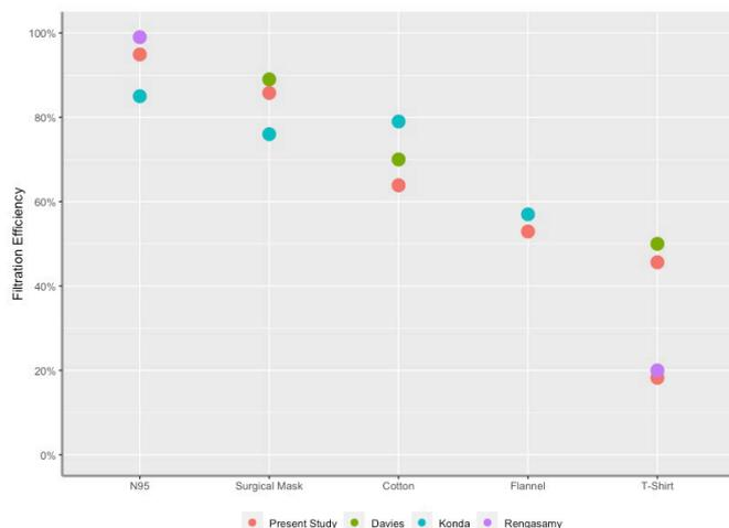
**Figure 3** A comparison of existing data on fabric ultrafine filtration. Data chosen represent the highest velocity for each study. Data from this study were adjusted to proportionally represent a velocity of 0.2 m/s for this comparison. Data from Rengasamy *et al*<sup>4</sup> are estimated from the included graphs, as statistical information about the data was not provided.
