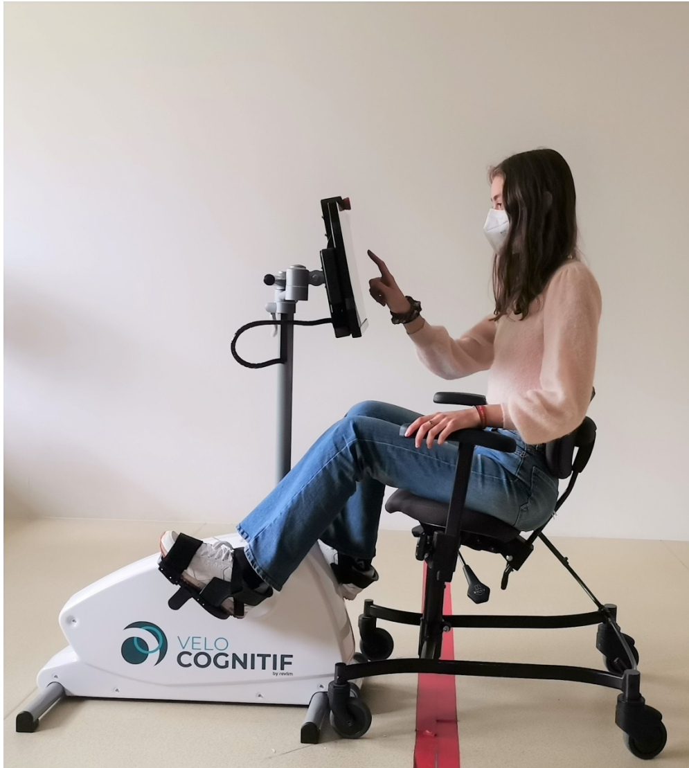
Figure 3. Vélo-cognitif (cognitive bike) consisting of an exercise bike to which a digital touch pad is attached to allow cognitive exercises to be performed while pedalling
