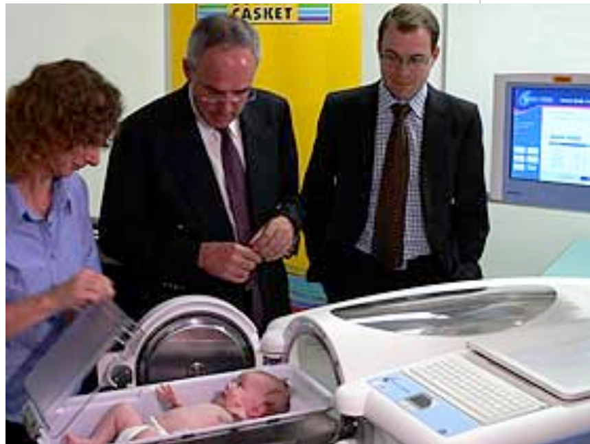
Life Measurement's Pea Pod air displacement plethysmograph assesses infant body composition. The top part of the machine enclosure is pressure formed by Freetech Plastics. The part measures 50-in. long by 32-in. wide. It features a large curved undercut all around the part and also has a molded-in recess to accept the blue inlay that serves as the bumper. At right is a rear view of the part showing added rib structures that were CNC machined before bonding.
