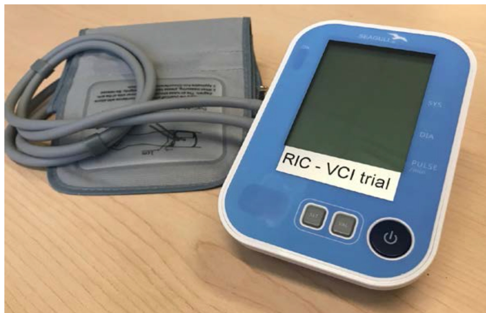
Figure 2. Device for applying remote ischemic conditioning (Seagull Aps, Denmark). The device applies four cycles of remote ischemic conditioning upon pressing the button. Device activations are recording, including the number of cycles. Systolic blood pressure, diastolic blood pressure, and pulse are displayed.
